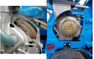
Conventional drill with rotating gear that "spills" seed into the drop tube (left panel), Precision planter with vacuum that picks up individual seeds and drops one seed at a time down the drop tube (right panel)
